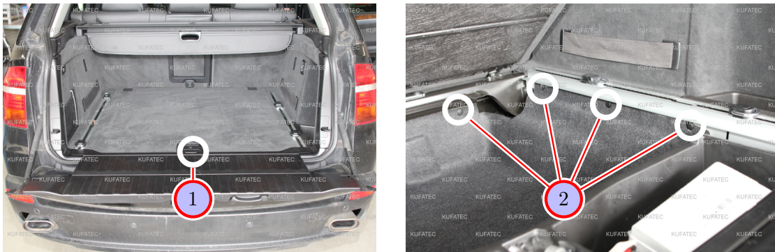
Figure 7: Disassembly coverings trunk
