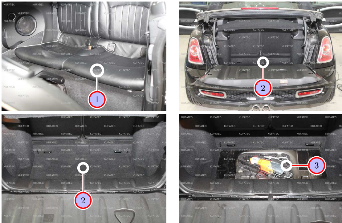
Figure 6: Removing back seats / trim panel trunk
